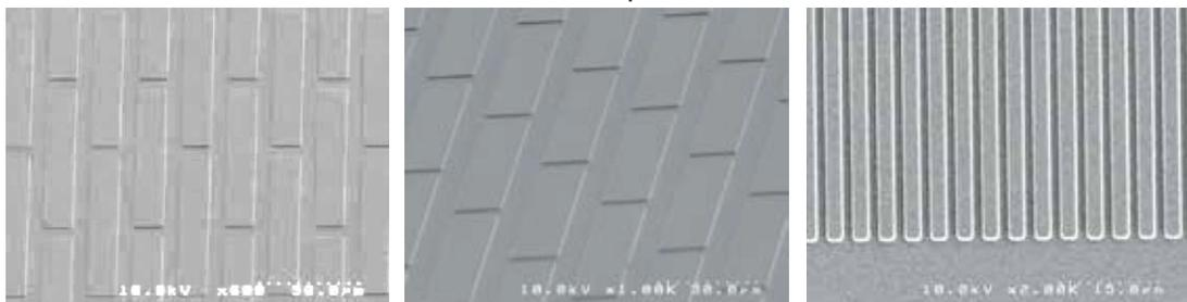
短辺幅30μm (400x280mm area)
